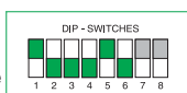
Figure 3: Example of setting address on Art. 1259C for control by means of code actuator 224
